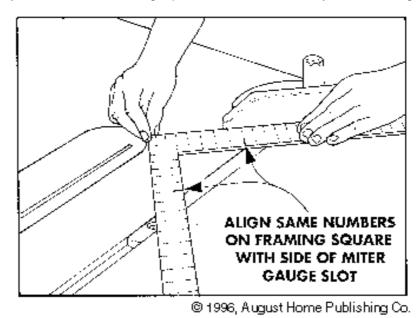
This technique gives you accurate mitres if the saw blade is parallel to the mitre gauge slot (which it should be).
